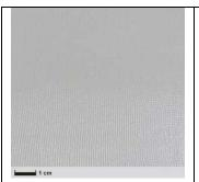
**RESIN CONSUMPTION:** 20G/M<sup>2</sup> LAMINATE THICKNESS: 0.027 MM, LAMINATE WEIGHT: 45 G/M<sup>2</sup>
