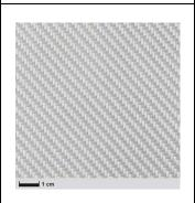
RESIN CONSUMPTION: 220G/M<sup>2</sup> LAMINATE THICKNESS 0.308MM / WEIGHT 500G/M<sup>2</sup>
