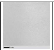
RESIN CONSUMPTION: 39G/M<sup>2</sup> LAMINATE THICKNESS: 0.050 MM, LAMINATE WEIGHT: 88G/MM
