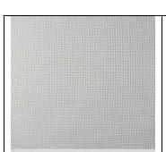
RESIN CONSUMPTION: 63G/M<sup>2</sup> LAMINATE THICKNESS: 0.088 MM, LAMINATE WEIGHT:143G/M<sup>2</sup>
