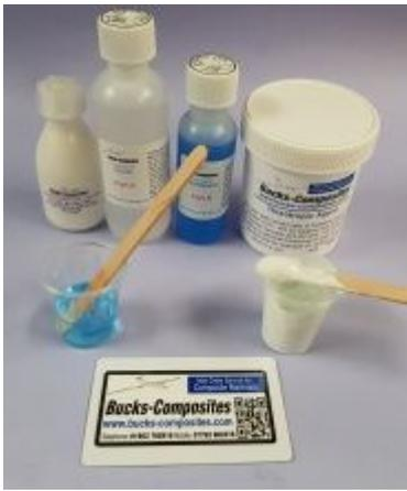
I have brushed a small amount of only the activated resin & hardener to the area where the activated paste will be added to increase the bond strength. I have used a plastic spreader card to smooth over the applied paste. I will leave to cure which normally takes 24 hours.
