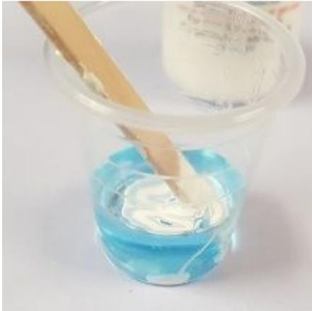
For this small repair I have measured out 10ml of resin and 5ml of hardener mixed well. I have poured 10ml of the activated resin & hardener into a pot and added a very small amount of the pure white colouring paste (a spatula just dipped into the colouring paste pot is enough) stirred well.
