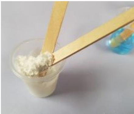
I have added the thixotropic agent to the coloured activated resin & hardener again stirred well to form a non drip epoxy paste for repairs. I have added the thixotropic agent until the mix stops flowing.
